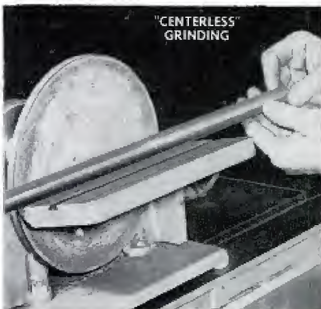
Polishing, or "centerless" grinding of steel shafting requires that the table be tilted up about 10 deg.
